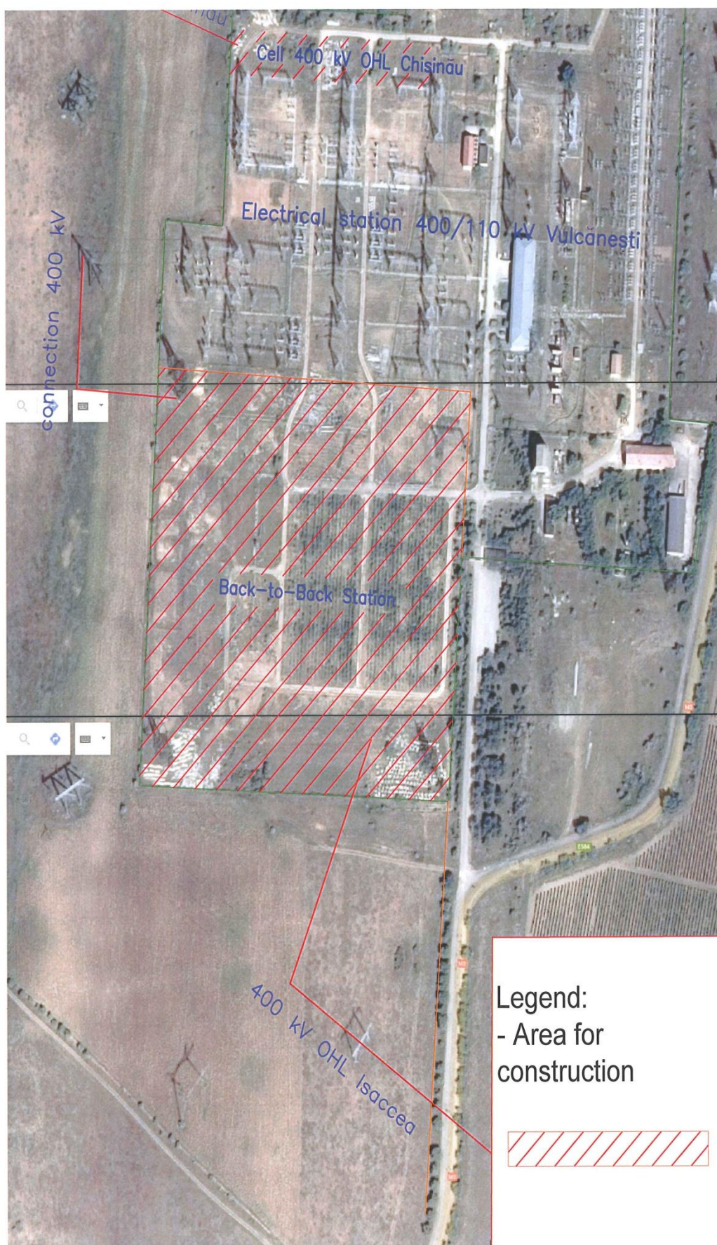
Figure 3.1.1.3 Vulcănești 400/110/35 kV sub-station and suggested area for construction of the “back to back” sub-station
